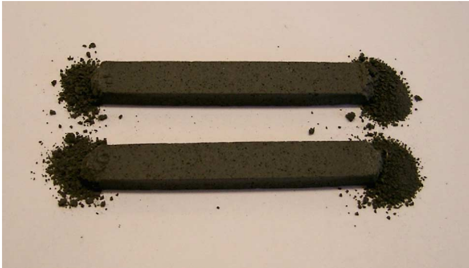
Fig. 4. Destroyed samples of SiC–Y 2 O 3 .
